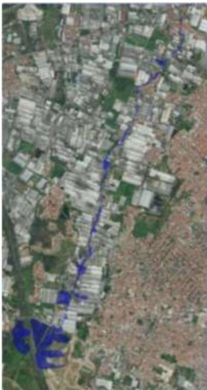
Fig. 14 Simulation with 125 000 m<sup>3</sup> Retention Pond for 2 year Return Period.
