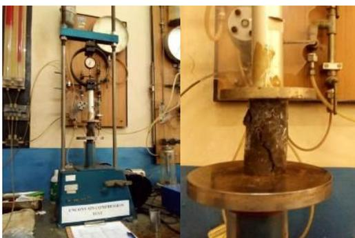
**Figure 2.** UCS Test
