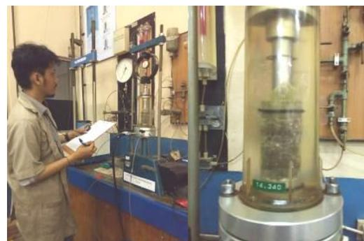
**Figure 3.** Triaxial UU Test
