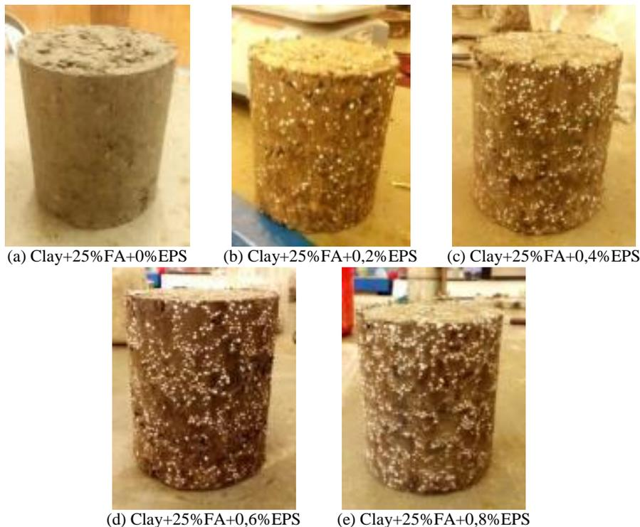
Figure 5. Extruded specimen of soil, 25% fly ash and varies content of EPS mixture
